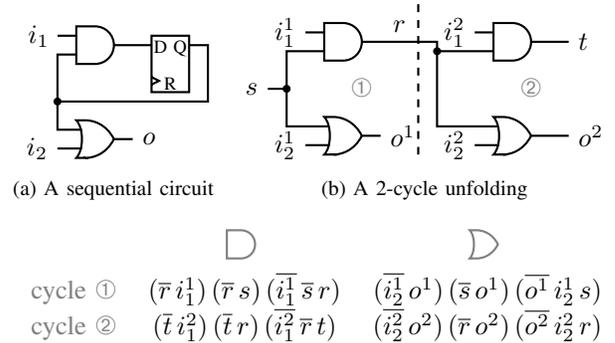
(a) A sequential circuit (b) A 2-cycle unfolding (c) CNF encoding of unfolded circuit. As usual, the operators  $+$  and  $\cdot$  are dropped for compactness. The clauses are grouped with respect to the gates and cycles by which they are contributed.
